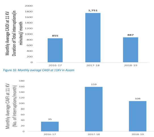
Figure 17: Monthly average CAIFI at 11KV in Assam (For interruptions exceeding 10 minutes at a time)
