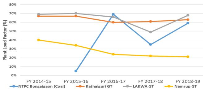
*Figure 9: Power Load Factor of thermal power plants in Assam over last 5 years Source: CEA*
